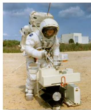
Jim Irwin (Apollo 15). The large black object at the bottom is the Radioisotope Thermoelectric Generator (RTG).
